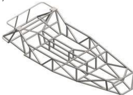
Fig 1. 3D modeling of tubular space frame
